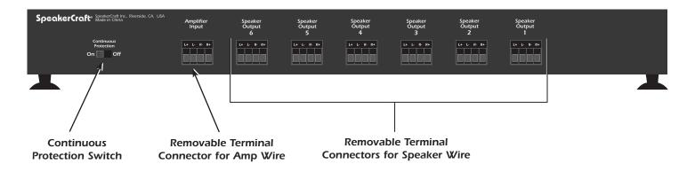
For best results, use speaker wire that is at least 18 gauge. For runs longer than 75 feet, 14 gauge wire is recommended. Wire larger than 14 gauge is not recommended because it may not fit into the connector. For best results, strip all wire insulation no more than 3/8" from the end before inserting into the connector.
