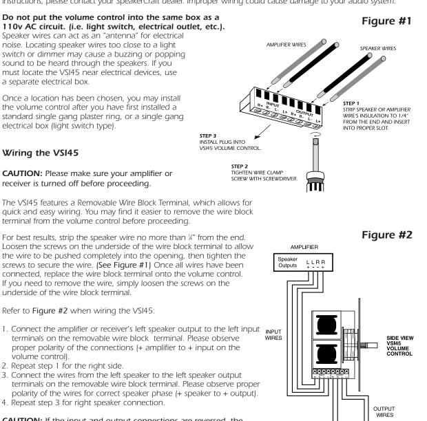
CAUTION: If the input and output connections are reversed, the minimum setting on the volume control will cause a short across the amplifier or receiver output terminals, resulting in serious damage to your amplifier or receiver. Please double check steps 1 through 4. This volume control cannot be connected in series with another volume control.
