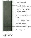
structure. A blend of sound-absorbent materials, the system prevents the sound from passing into the drywall, dampens drywall resonance, halts standing waves and Helmholtz resonance, and dissipates back-waves. The result? New power and definition at the bass end.
