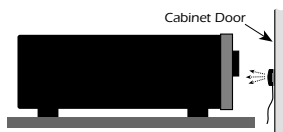
Fig. 5b IRE-1.0 attached to inside of cabinet door directly opposite IR sensor window
