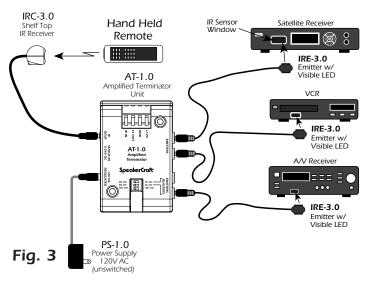
**Note 4**: The emitter shell and EZ-Docker port, though dark in appearance, are transparent to Infrared. This allows IR commands to pass through them, permitting local hand held remote control as well as through the IRE-3.0.
