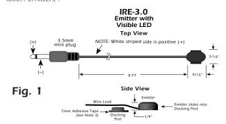
**ATTACHMENT** First, locate the component's IR Sensor window (See Note 1) and thoroughly clean it of any fingerprints or other greasy substances The EZ-Docker" port has a clear adhesive layer on its bottom surface.
